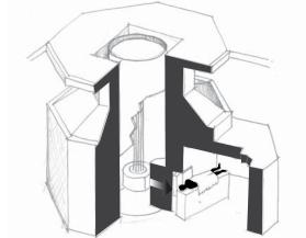
The TRIGA research reactor at VTT in Finland has been in operation since 1962. The uranium fuel is enriched to 20 % and it is moderated by light water. The power output is 0,25 MW. The present operation is mainly for Boron Neutron Capture Therapy.
