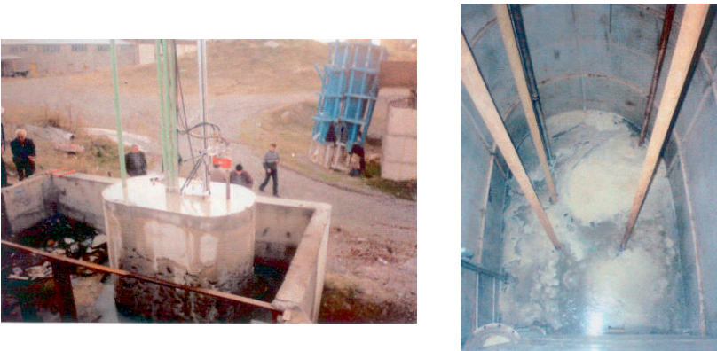
FIG. 9. Mock-up of grouted IRT reactor in Georgia.
