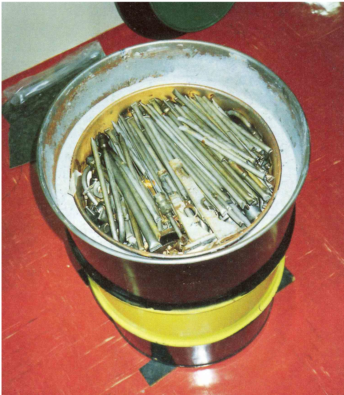
Figure 7-5. Drum packed with steel pipes and other metallic objects.
