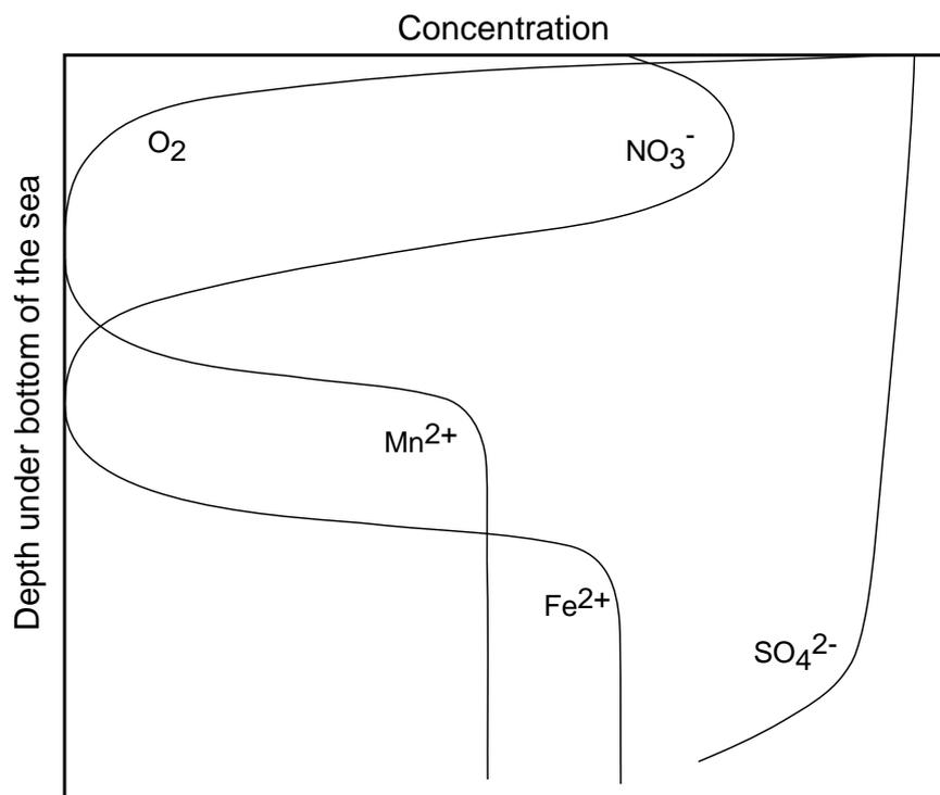
Figure 3. Oxidation of sea sediments. The bacteria usually prefer free oxygen. Nitrate formed in the decomposition can however diffuse further into the seabed than the oxygen (cf text). In the absence of oxygen, manganese may be reduced, and at lower redox potential also iron. At the lowest redox potentials, sulphate can become reduced in which case sulphur or hydrogen sulphide is formed. After (Burdige, 2006).
