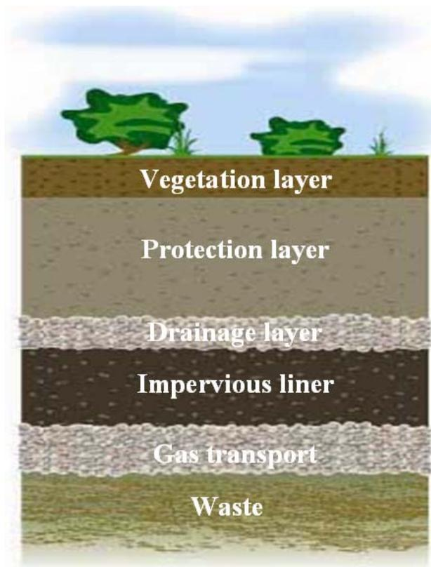
Figure 1. The generic design for covers at the Landfill Site at the Tveta Recycling Plant.
